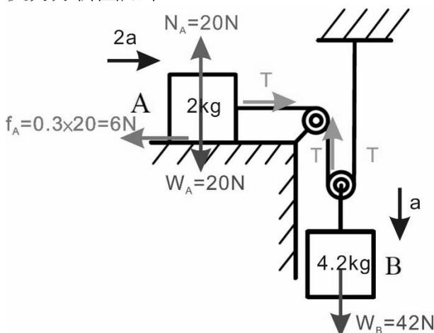
$$(1) \begin{cases} \text{分析A: } T - 6 = 1 \times a \\ \text{分析B: } 42 - 2 = 4.2 \times a \end{cases} \Rightarrow \text{解 } a = \frac{2.46\text{ m}}{\text{s}^2}$$
